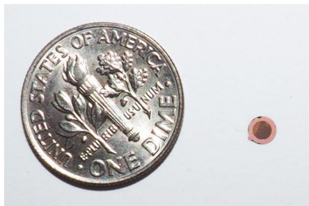
“Breakup” foils (originally for electron microscopy). Thickness \sim 3\text{-}4\text{nm}
