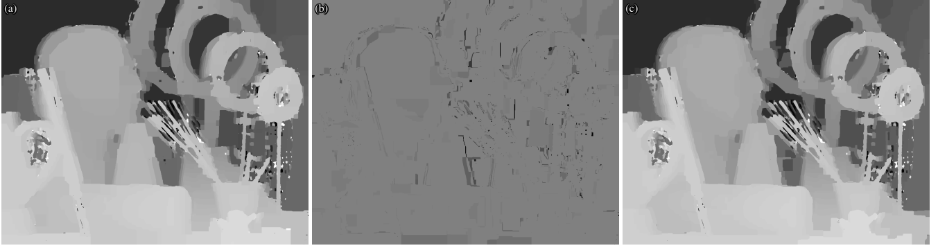
Figure A.4: Depth map resulting from optimization of the Planesweep_1280_1022_96 dataset for (a) GCO and (c) our solver. (b) shows the difference image (a gray value of 128 corresponds to a difference of 0).
