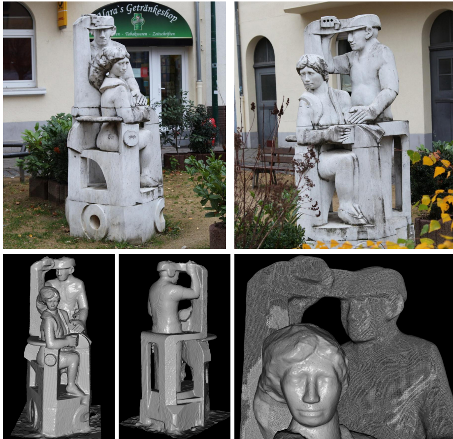
Fig. 12. Two input images of the Kopernikus data set, the complete reconstructed model from two perspectives and a close-up of the wireframe showing the adaptively triangulated mesh.
