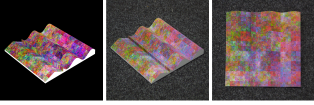
Figure 4. Left : Rendering of the test target. Middle/Right : Side and top view of the manufactured test target.
