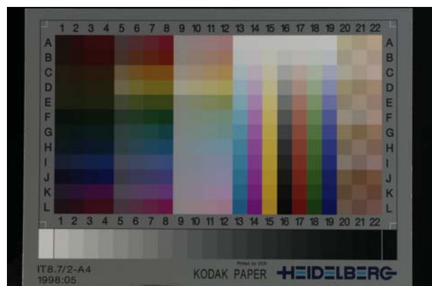
Figure 3: Image generated from the HDR image of the IT8 target.
