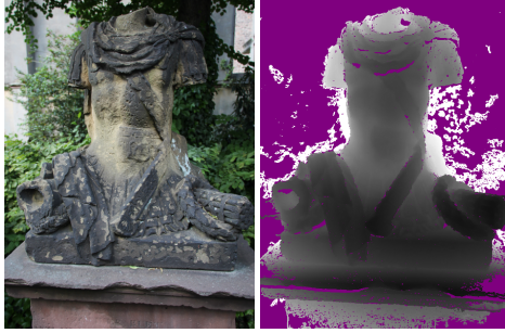
Figure 4: An input image and the corresponding depth map reconstructed with multi-view stereo. Each depth value encodes the distance from the camera.
