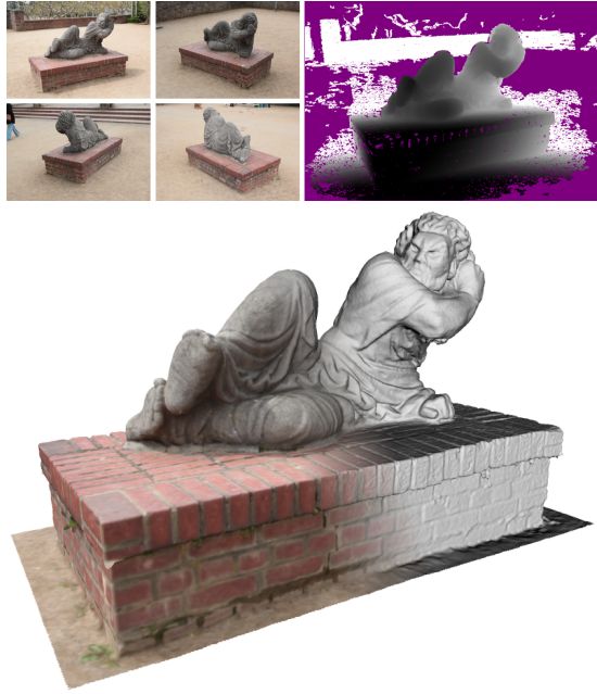
Figure 11: The Der Hass dataset. The top row shows 4 out of 79 input images and a depth map. The bottom row shows the reconstruction with color (left) and shaded (right).
