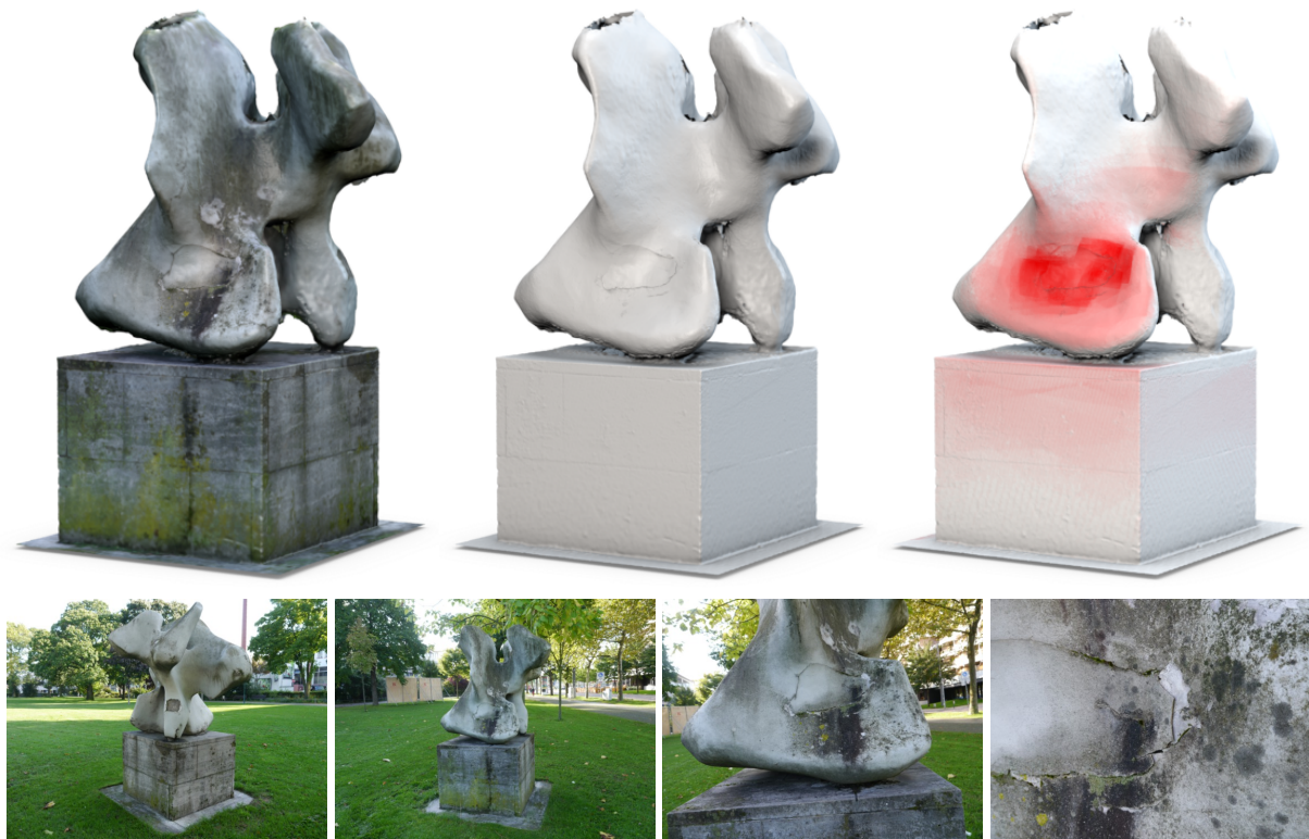
Figure 2: Multi-scale reconstruction of the Sculpture dataset. The first row shows the reconstruction with color (left), with shading (middle) and with false coloring of the scale. The bottom row shows 4 of 120 input images with varying scale.
