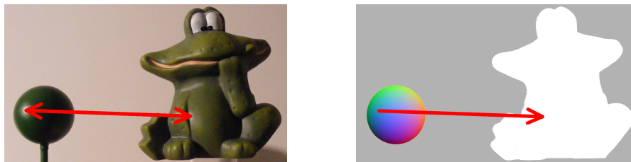
Figure 7.2: The concept of appearance matching for shape reconstruction. Left: Finding pixels with similar intensity (usually in a series of images) on the target and a reference sphere. Right: Because of orientation consistency, normals can be transferred between matches.
