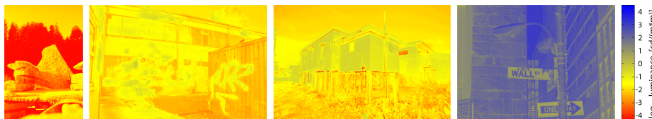
Fig. 7. Colormapped \log_{10} of absolute luminance. Images from left to right correspond to rows in Fig. 5 and Fig. 6. The respective logarithmic mean of estimated luminances is: 0.0003 \text{ cd/m}^2 , 0.014 \text{ cd/m}^2 , 0.018 \text{ cd/m}^2 , 92.86 \text{ cd/m}^2 . The estimated luminance factor is: 0.087 \text{ cd/m}^2 , 0.576 \text{ cd/m}^2 , 0.407 \text{ cd/m}^2 , 1128.23 \text{ cd/m}^2 .
