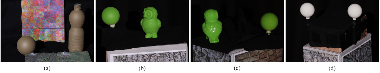
Figure 6. Datasets with varying reflectance. (a-d) Cropped input images for the bottle , diffuse owl , shiny owl , and spheres datasets corresponding to the depth and normal maps shown in Section 5. We use the textured patterns in each scene to estimate camera pose.
