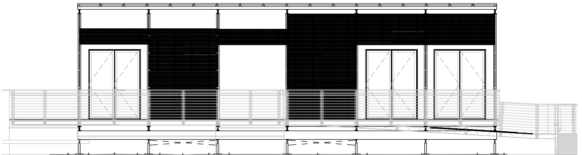
North elevation with screens (open position)
