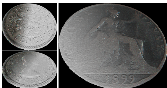
Figure 7: Reconstruction of shiny objects without treatment (blending between textured and gray-scale shaded rendering). Left: Sixpence coin from 1955, front and back. Right: One Penny from 1899.
