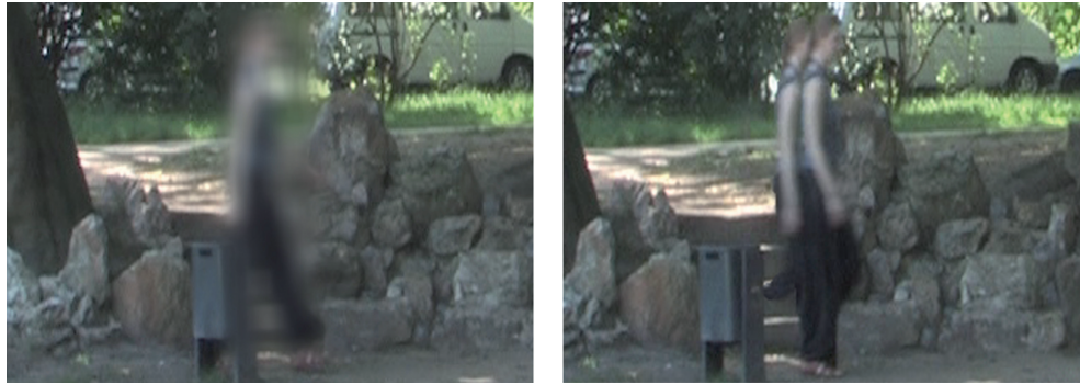
Fig. 3. Example of two artifacts shown in the videos, left: blurring on person, right: ghosting.
