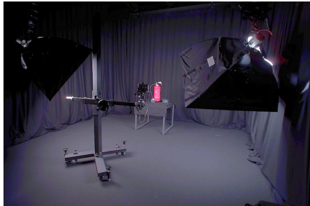
Figure 3.1: A view of our photo studio with black, diffuse reflecting material on the floor, walls, and ceiling. This image was generated from a High Dynamic Range image to which a tone-mapper has been applied.
