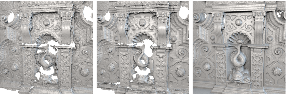
Fig. 6. The fountain-P11 dataset from Strecha et al. [32]. From left to right: Reconstruction by our implementation of Semerjian [5] using a low regularization weight to recover details; by our new optimization; and ground truth.
