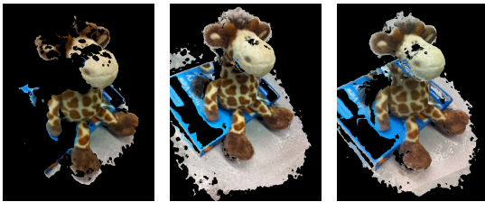
Figure 6: Left : Multi-view stereo reconstruction with just the initial set of images. Middle : Final reconstruction with 22 images. Right : Reconstruction from a dataset of 22 images captured by an expert without explicit view planning.
