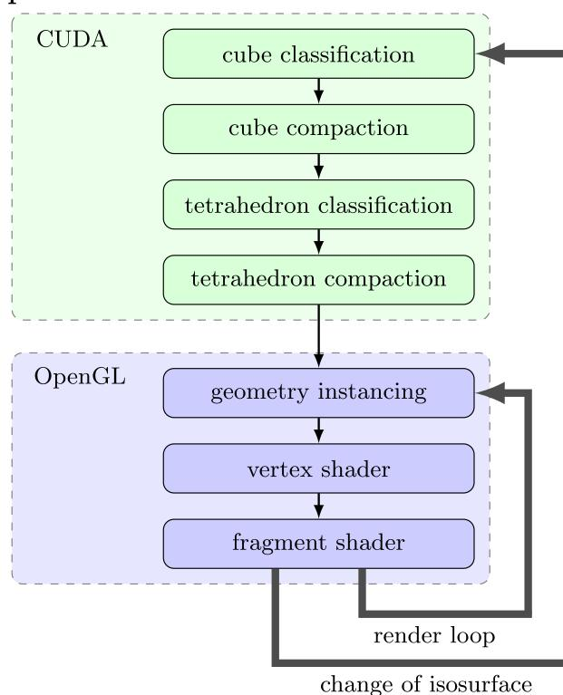
The CUDA kernels are invoked for each change of isosurface:
