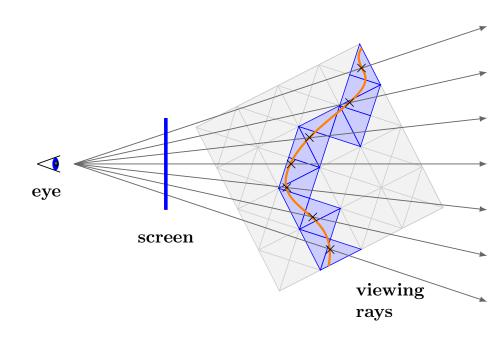
Visualization is done in a hybrid rasterization / ray casting approach where we use instancing to draw the bounding geometry.
