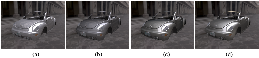
Figure 7: Comparison renderings using different BRDFs for the car body in the same lighting. a) Phong. b) Industrial state of the art car paint model (based on the ClearCoat™ model). c) Our measured car paint BRDF. d) Our fitted BRDF model. Note the different distribution of reflection intensity in the Phong example, and the different placement and shape of the highlights in the ClearCoat™ example. Also note that the fitted BRDF matches the tabulated BRDF well and completes the missing data at grazing angles.
