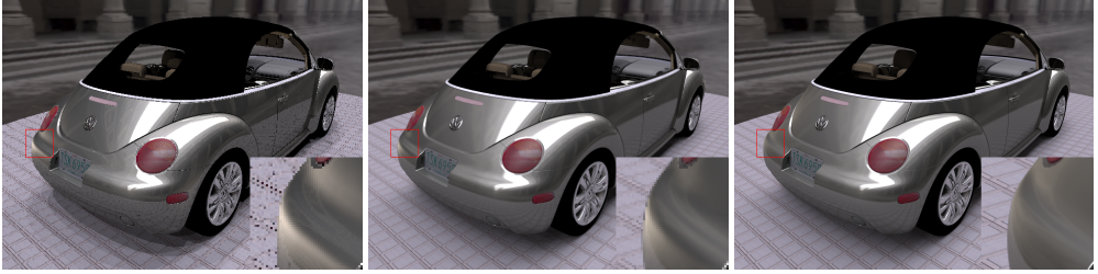
Figure 8: Comparison of renderings with different quality settings generated by 20 dual Opteron 2.5 GHz PCs. Left: Low quality settings (light sources l = 16 , specular lobe samples s = 1 , samples per pixel p = 1 ) to gain realistic frame rates of 12.1 fps. Note the visible shadow boundaries, the aliasing artifacts as well as the unrealistic sharp reflections. Center: With medium quality settings ( l = 128, s = 16, p = 16 ) most of the aliasing artifacts already vanished. The performance of 1.3 fps still allows for interacting with the model. Right: High quality settings ( l = 1024, s = 256, p = 64 ) are used for offline rendering (97 seconds) at a high resolution of 1280 \times 960 .
