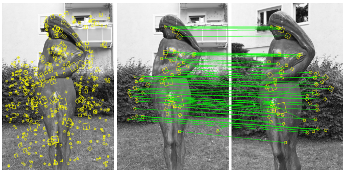
Figure 3: Feature detection (left) and feature matching between two views (right). The horizontal lines are mostly good matches, while the heavily slanted lines are outliers. Enforcing two-view constraints will remove most outliers.
