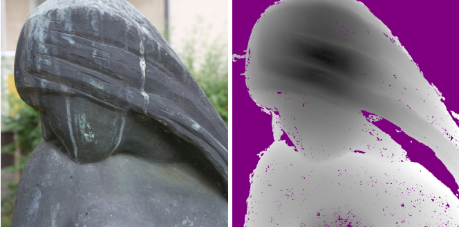
Figure 5: One of the input images and the corresponding depth map reconstructed with multi-view stereo. Each depth value encodes the distance from the camera center to the geometry.
