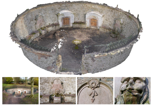
Figure 16: The Fountain dataset. The top row shows the full colored reconstruction of the site. The bottom row shows 4 of 384 input images depicting the whole site, the fountain and two details on the fountain.
