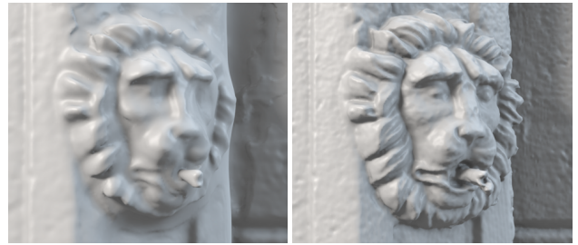
Figure 19: Comparison of reconstructions using signed distance ramps (left) and our basis function using Gaussians (right). The distance ramps are particularly harmful in mixed-scale datasets.
