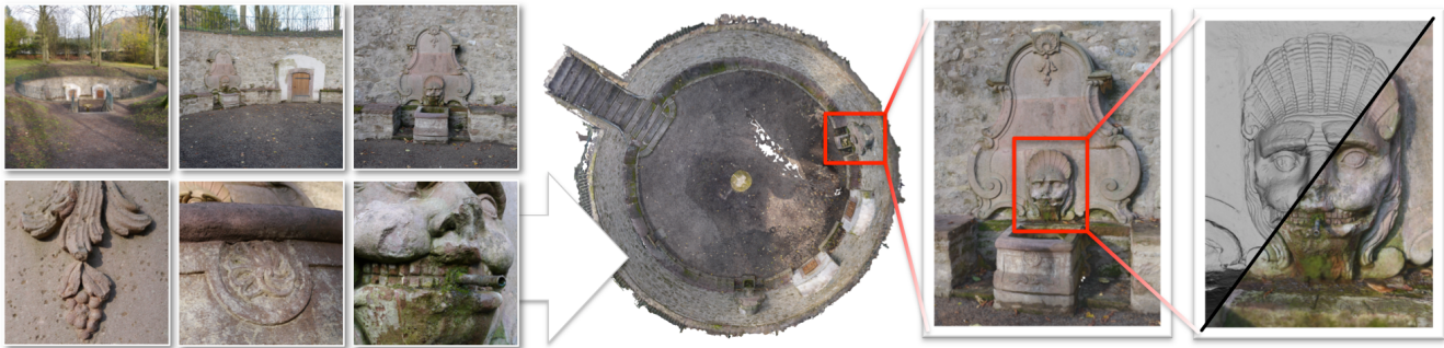
Figure 1: Floating Scale Surface Reconstruction example. 6 out of 384 input images of a multi-scale dataset (left). Registered images are processed with multi-view stereo which yields depth maps with drastically different sampling rates of the surface. Our algorithm is able to accurately reconstruct every captured detail of the dataset using a novel multi-scale reconstruction approach (right).
