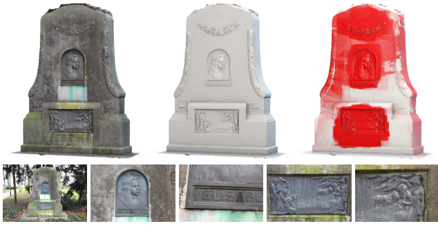
Figure 14: Multi-scale reconstruction of the Elisabeth dataset. The top row shows our reconstruction with color (left), with shading (middle) and with false coloring of the scale (right). The bottom row shows 5 of 205 input images with varying scale.
