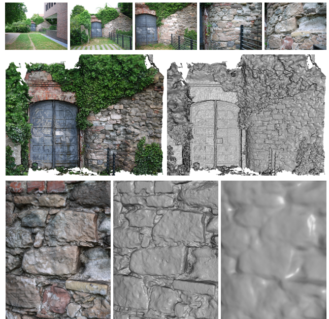
Figure 10: The top row shows some input images from the Stones dataset, and the middle row shows the reconstructed scene. The bottom row shows a close-up view of our reconstruction with and without texture (left, middle), and the corresponding VRIP reconstruction (right).
