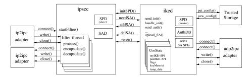
**Fig. 3.** Schematic overview of the iked and ipsec security modules and IPC channels. Arrows indicate the possible direction of a call, order of calls represents a possible session flow for that interface. The iked component creates a *ConState* structure for each handshake attempt and maintains a list of active SPIs.
