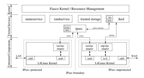
**Fig. 2.** Detailed architecture of sVPN. A single platform acts as a VPN gateway with two physical network interfaces. The "protected" compartment routes plaintext traffic between the LAN and sVPN. The "unprotected" compartment is responsible for routing the secured data streams into the WAN.
