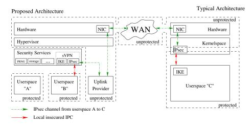
**Fig. 1.** Overview of the sVPN architecture interfacing with a commodity IPsec implementation through WAN/Internet. The sVPN security service processes all data passing through a local channel between "B" and the "Uplink Provider", according its IPsec policy. By applying IPsec protection to some of the data streams, local channels are logically extended into secure remote channels that reach through the unprotected area to a peer IPsec gateway.
