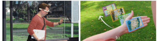
Figure 1. A map application as an example of one-handed (a) proximity-based interaction with a linear layered information space. The user can access different map layers by moving his hand through the space (b).
