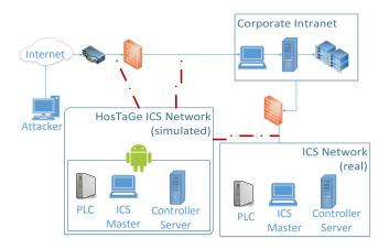
Fig. 1: HosTaGe network positions architecture
